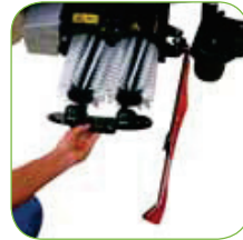
Combined scrubbing-sweeping system that includes debris hopper (CT230 R Sweep).
